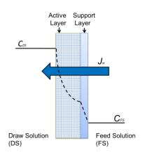
Figure 1: Principle of forward osmosis
