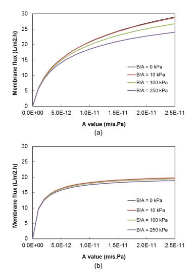
Figure 2: Effect of membrane active layer properties (*A* and *B*) on FO water flux. (a) Wastewater treatment scenario and (b) seawater desalination scenario. Other simulation conditions include S = 0.4 mm and  $D = 1.69 \times 10^{-9}$  m<sup>2</sup>/s.
